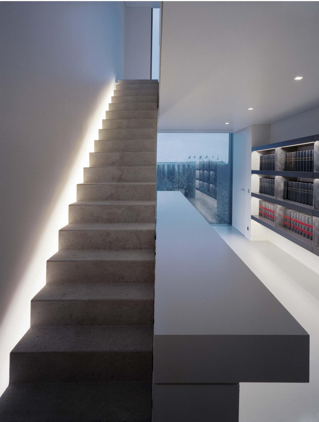
**concept:** in order to underline the minimalistic architecture, the lighting scenography is based solely on the use of deeply recessed lighting fittings. two independent lighting schemes were developed: indirect lighting to emphasize the architectural features (concrete bench and staircase) and direct lighting for the task and representation functions (by means of discrete down lighters).
